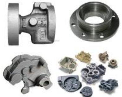
This would be a suitable method of manufacturing for my product because it has a low set up cost. This means that it would be suitable for batch production. Aluminium can be sand cast into complex shapes. However it will also mean that I have to spend a lot of time finishing the parts after I have sand cast them.
